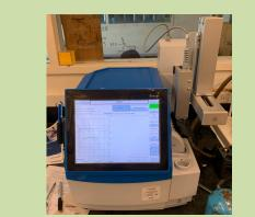
Samples placed in the microwave digester for 10 minutes at 180°C
