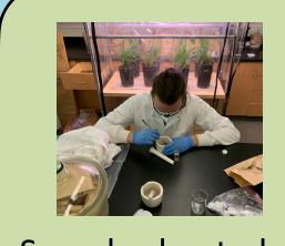
Samples heated at 75°C until dry and ground to a fine powder
