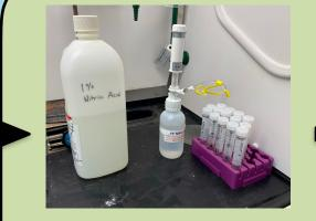
Samples filtered into a falcon tube and diluted to 10 mL with 1% HNO<sub>3</sub>
