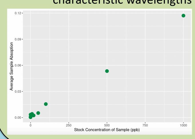
Zn standard curve, detection limit < 50 ppb
