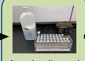
Samples digested for 12 hours with 500 μL of 70% metal free HNO<sub>3</sub>
