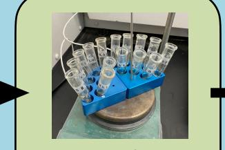
500 μL of H<sub>2</sub>O<sub>2</sub> added to samples and set on 50°C hot plate
