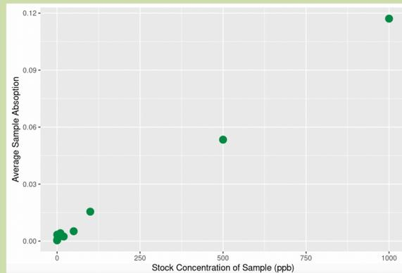
Zn standard curve, detection limit < 50 ppb
