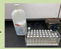
Samples digested for 12 hours with 500 µL of 70% metal free HNO<sub>3</sub>
