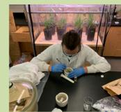
Samples heated at 75°C until dry and ground to a fine powder
