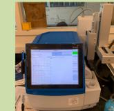
Samples placed in the microwave digester for 10 minutes at 180°C
