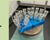
500 µL of H<sub>2</sub>O<sub>2</sub> added to samples and set on 50°C hot plate
