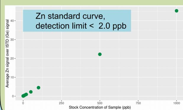
Zn standard curve, detection limit < 2.0 ppb
