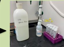
Samples filtered into a falcon tube and diluted to 10 mL with 1% HNO<sub>3</sub>
