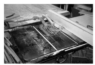
Table saw equipped with self-adjusting blade guard.
