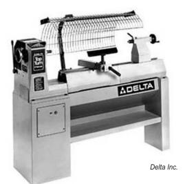
Make sure the tool rest is secure and set close to the stock (1/8-inch). Rotate the stock by hand to make sure it clears the tool rest before turning the lathe on. Guide the turning tool on the rest only — do not attempt to support the tool with your hands.
