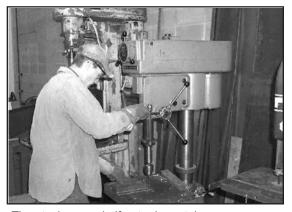
The stock can spin if not adequately secured to the table.
