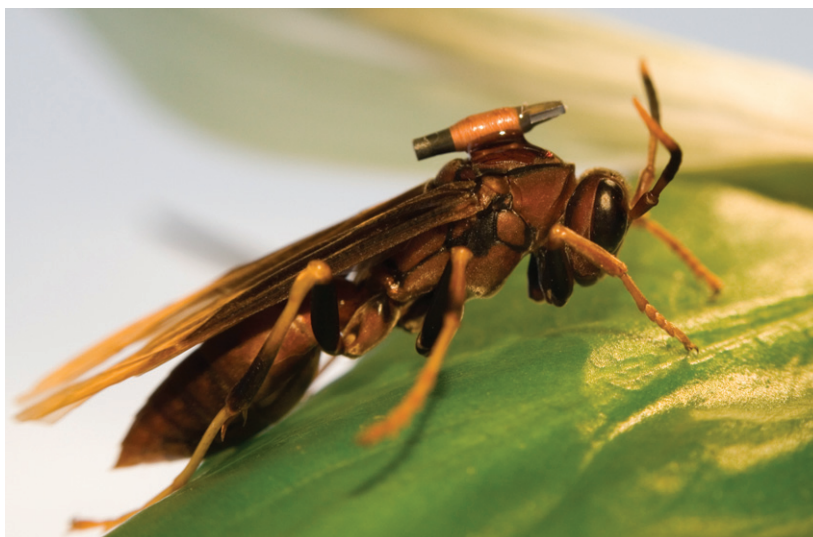
Figure 6 A paper wasp tagged with a passive RFID. The tag shown is an insert of a PIT tag, without the outer glass casing. Photo by Aidan Weatherill.
