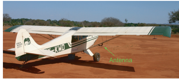
Figure 3 Light aircraft with antennas connected to each wing for wildlife tracking. Photo by Roy Wollman.
