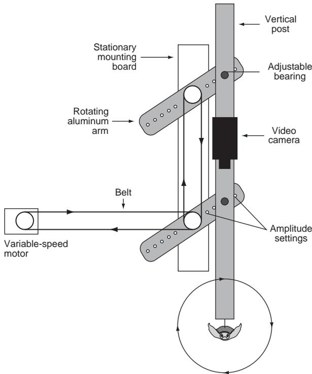
**Figure 2** A machine designed to simulate wave motion by reproducing the sequence of accelerations that occur beneath a propagating wave. The responses of hatchling turtles to these simulated waves have been studied by placing turtles into cloth harnesses and subjecting them to orbital movements while they are suspended in air. Modified from Lohmann KJ, Swartz AW, and Lohmann CMF (1995) Perception of ocean wave direction by sea turtles. *Journal of Experimental Biology* 198: 1079–1085.
