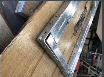
I used 2"x2" aluminum rods to create a ladder like support underneath the plank, upon which was attached the hardware needed to connect a crossbeam
