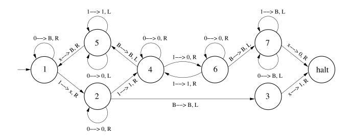
Figure 1.5: The state diagram of the power-of-2 decision Turing machine  $M_{pow}$
