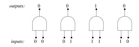
Figure 2.1: The AND gate computes  $x \wedge y$
