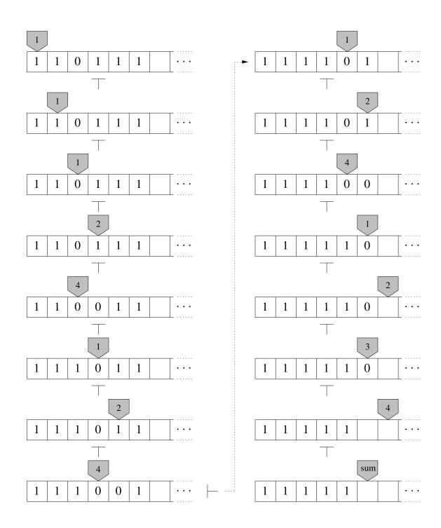
Figure 1.7: Configurations of the Turing machine  $M_{sum}$  on a string 110111
