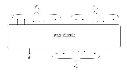
Figure 3.4: The state component for an arbitrary Turing machine
