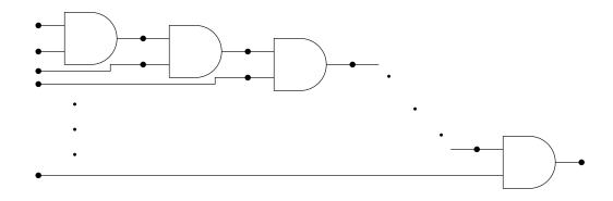
Figure 2.6: A connection of n AND gates
