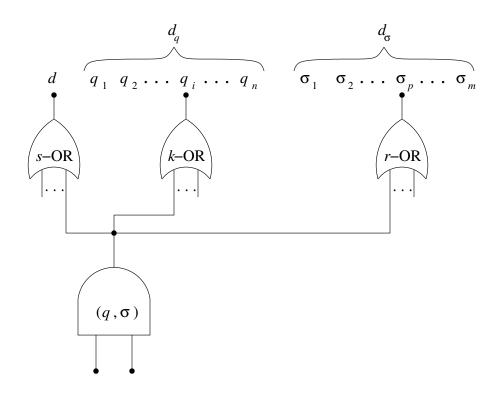
Figure 3.13: An output where  $\delta(q, \sigma) = (q_i, \sigma_p, L)$
