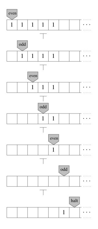
Figure 1.3: Configurations of the parity-decision machine on a string 11111
