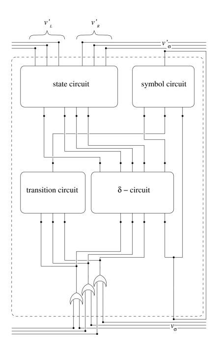
Figure 3.9: The cell circuit for  $M_{odd}$
