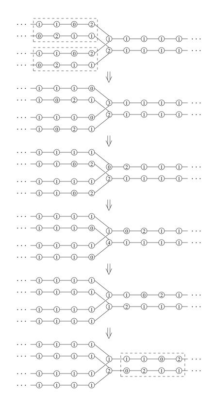
Figure 4.12: The sandpile AND-gate evaluates  $1 \wedge 1 = 1$
