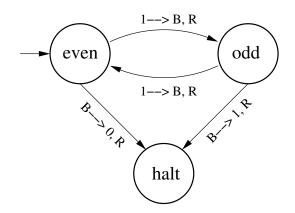
Figure 1.2: The state diagram of the Turing machine  $M_{odd}$
