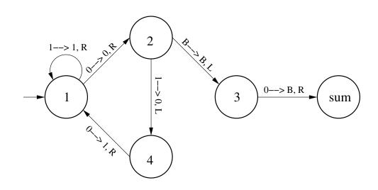
Figure 1.6: The state diagram of the sum-computing Turing machine  $M_{sum}$
